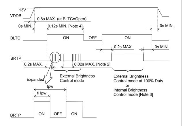
[Note 1] External PWM duty DBRTP = tHpw / tpw : 30 - 100 % External PWM frequency FBE = 1/tpw : 50 - 300 Hz
