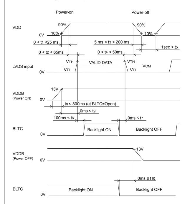
When the VDD is off, LVDS input must be kept at either low level or high impedance.
